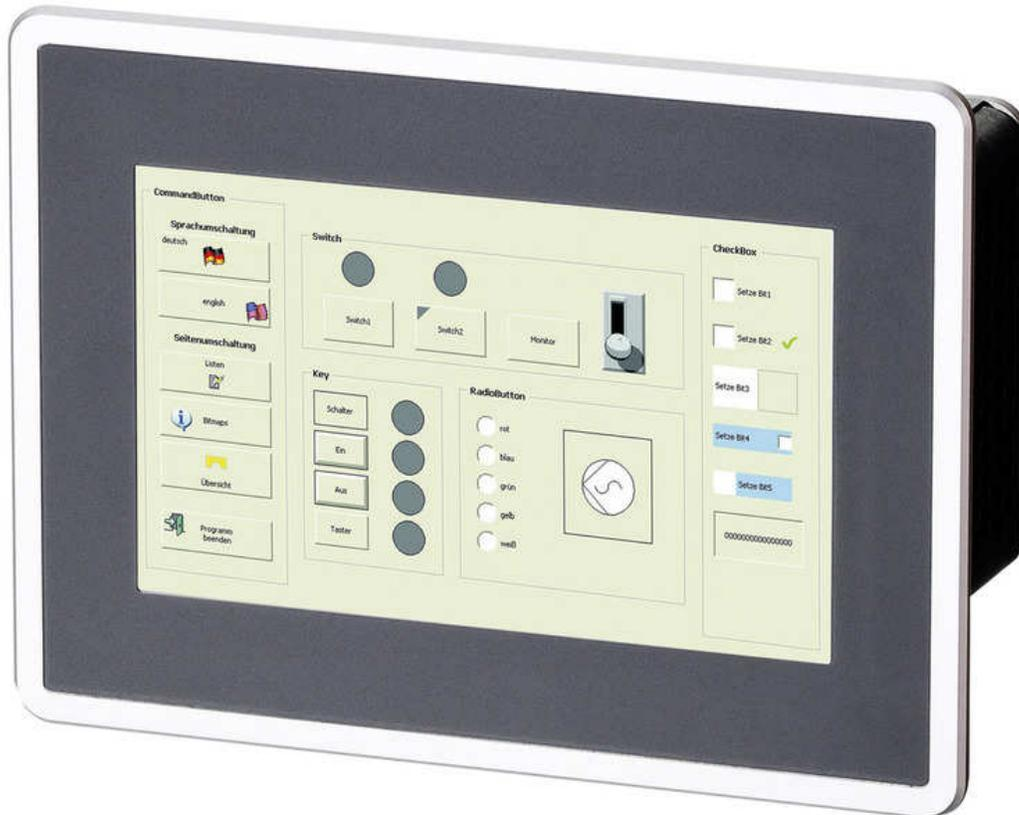
Panel controller p300 combines logic (PLC) and visualization in a compact device and is ideally suited to machine applications which only require a low processing power. With the same system properties as its older brother, its strength lies in its visualization capabilities when used as an HMI. By extending the Controller portfolio with the p300, Lenze has opened up new possibilities within the system.
