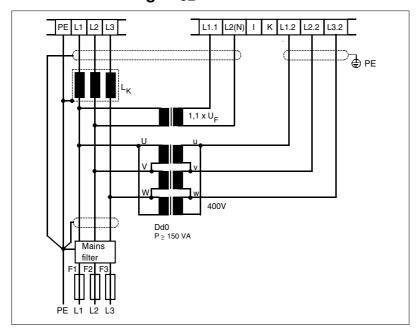
If the mains voltage is lower than 340 V the control electronics must be supplied separately via the step-up transformer as shown in the illustration.
